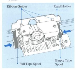
• Make sure that the inner surface of the tape on the spool faces toward the Platen.
