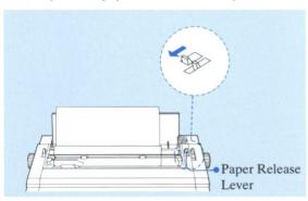
3 Return the Paper Release Lever and Paper Bail Lever to their original positions and then position the Paper Bail Rollers to hold down the paper.
