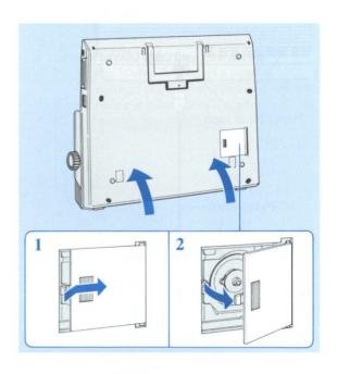
5 Grasp the Lever of the Cupwheel Printing Element between your fingers to release the lock. Then pull it directly out as shown in the figure.
