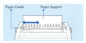
Insert the paper straight under the back of the Platen.
