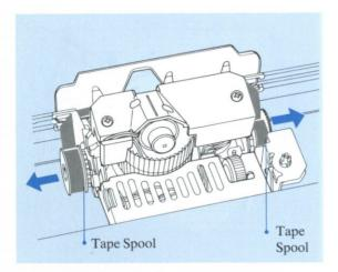
3 Place the new Correction Tape with the Full Spool on the left side, and then pass the tape between the Card Holder and the Ribbon Guides.
