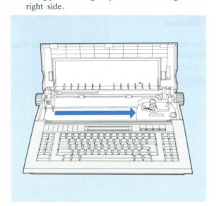
4 Close the Top Cover again and place the Typewriter on its back. Remove the Bottom Cover Lid by sliding it to the right side.
