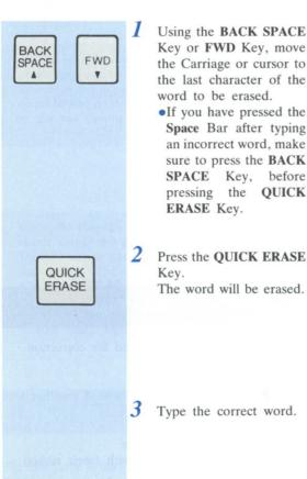
By pressing the QUICK ERASE Key when the Carriage or cursor is in the middle of a word, the characters to the left of the current position will be corrected.
