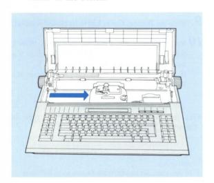
Turn the Ribbon Feed Wheel (on the new Ribbon Cassette) clockwise to tighten the Ribbon.
