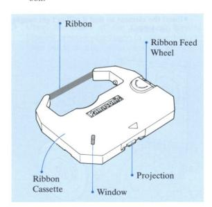
Position the new Ribbon Cassette over the Cassette Holder so that the Window (through which the ribbon can be seen) is on the top, then place the Projection on the rear of the cassette into the Slot at the front of the Cassette Holder.
