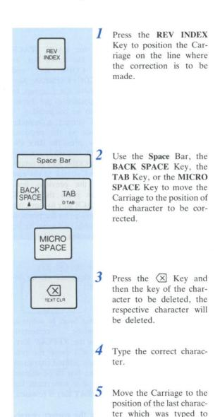
To manually erase a character printed in the "PS" pitch, first align the Carriage with the character using the MICRO SPACE Key.
