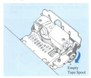
5 Install the Ribbon Cassette properly. (Follow the steps 5 through 8 of "REPLACING THE RIB-BON CASSETTE".)
