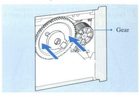
8 Hold the Knob of the Cupwheel Printing Element and turn it slightly to check that it rotates freely.
