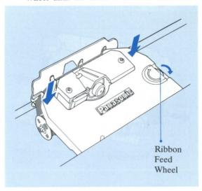
8 Confirm that there is no slack in the Ribbon. If there is slack, turn the Ribbon Feed Wheel clockwise to remove it.
