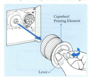
•If a Cupwheel Printing Element without the Lever is used, grasp its Knob and pull it directly out.
