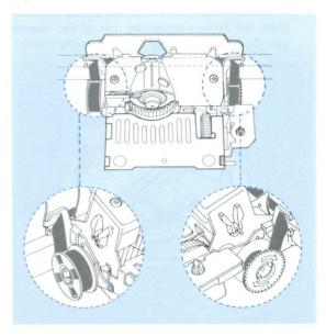
4 Turn the right spool clockwise until the white tape appears at the center of the Card Holder.
