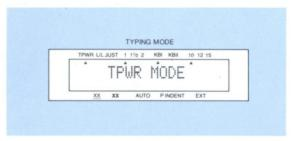
If the "▼" mark appears above "EXT" at the bottom right of the LCD Display, press the CODE Key and then press the 8 Key at the same time to delete the "▼" mark.
