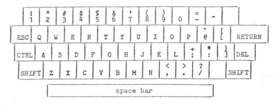
The CTRL key is used like a shift key to send the CONTROL CHARACTERS, control-A through control-Z. To type a control character, hold the CTRL key down while typing the letter. In this manual, "control" is abbreviated ""; that is, "A means control-A, typed by holding down CTRL and typing an A; "B means control-B, etc. Control characters are used for COMMANDS to WordStar, to tell WordStar to do something; other keys enter document characters.
