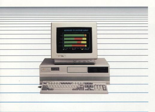
The advanced 32-bit 80386 microprocessor brings supermini performance to this desktop PC...it's the next generation of power and speed.
