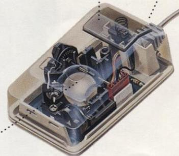
*The inside story — a rotating ball and optical sensors translate movements of the mouse to Macintosh's screen pointer with pin-point accuracy.*
