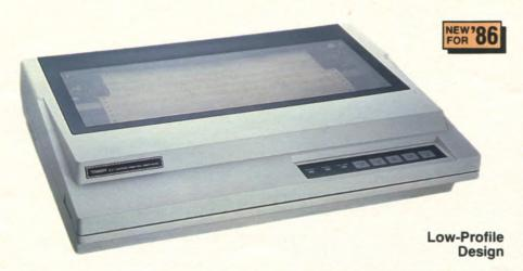
SPECIFICATIONS. Print Density: 10, 12, 17.1 (standard); 10 and 12 (correspondence); proportional and compressed proportional. Print Speed: Standard 10 cpi—380 cps. Correspondence 10 cpi—90 cps. Proportional—77-180 cps. Character Set: 95 ASCII, 31 graphics and special characters. IBM Character Set 1 and 2. Horizontal Dot Resolution: 60-240 dots/inch, 1632-3916 dot columns/ line. Dimensions: 43/a x 22/t/z x 167/k" Weight: 393/a lbs. Power: 120VAC, 60 Hz. 200W.
