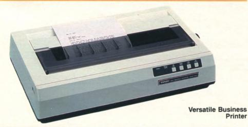
SPECIFICATIONS. Print Density: 10, 12, 16.7, proportional-spaced, elongated and condensed. Print Speed: Standard 10 cpi—93 lpm/80 col., 60 lpm/132 col. Correspondence 10 cpi—700 + wpm. Character Set: 96 ASCII, plus selectable Tandy standard, .64 special and 30 block graphics characters, or full 128-character Model 2000/IBM set. Horizontal Dot Resolution: 60-240 dots/inch, 1584-2640 dotcols./line. Dimensions: 43/4 x 227/16 x 133/4.\* Weight: 271/z lbs. Power: 120VAC, 60 Hz, 100W.
