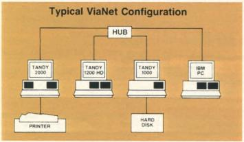
Most important, all of these operations are entirely transparent to users. Operating system commands work precisely the same under ViaNet as in a stand-alone environment. Each computer in the system requires a user-installable Arcnet Datalink Board, and is connected to a "hub" with coaxial cable. Boards include software and user's guide. Installation recommended (not included). ViaNet requires 128K more RAM than is required for applications and MS-DOS.
