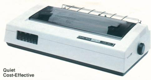
SPECIFICATIONS. Print Speed: Standard 10 cpi-181 lpm/20 col., 126 lpm/40 col., 78 lpm/80 col., 51 lpm/132 col. Correspondence 10 cpi-705 wpm. Character Set: 96 ASCII, 32 special and 30 block graphics characters. Pin Wire Diameter: 0.30mm. Horizontal Dot Reso
