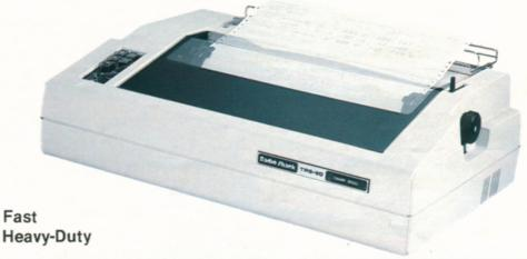
SPECIFICATIONS. Print Density: 10, 12 or 16.7 cpi in 9×9, 15×9 or n×9 (n = 1-23) dot matrix. Character Set: 96 ASCII, 32 special and 30 graphics characters. Pin Wire Diameter: 0.30mm. Horizontal Dot Resolution: 60-100 dots/inch, 792-1320 dots/line. Line Feed: 1/6, 1/8, 1/72, 1/216". Dimensions: 711/16×245/8×157/8". Weight: 50 lbs. Power: 120VAC, 60 Hz, 180W.
