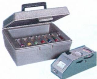
Use the multi-purpose Dip Meter to find approximate resonant and operating frequencies of either energized or de-energized circuits. The HD-1250 helps adjust traps, detect parasitic oscillations and harmonics, measure unknown Q/L/C values, locate sources and frequencies of RF energy. Use too as a signal generator, relative field strength meter or receiver alignment tool. Requires 9V battery. 2" H x 2 1/4" W x 5 7/8" D.
