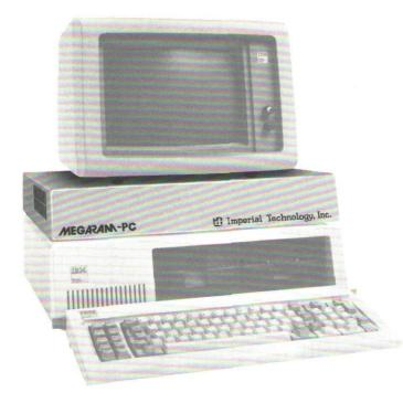
The MegaRam-PC storage system is a solid-state, nonrotating memory system which is interfaced to the computer as if it were a rotating disk.
