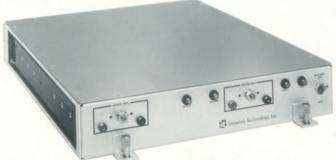
The battery back-up option consists of an optional power supply assembly which replaces the standard assembly inside the MegaRam chassis. This optional supply contains a battery pack capable of supporting a full 40 megabyte capacity MegaRam system for approximately 10 minutes. Additional support time can be obtained by adding external batteries.
