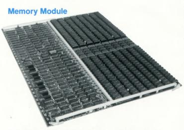
The MegaRam memory module is a semiconductor module employing 256Kxl dynamic MOS integrated circuits. The capacity of the module is 8,388,608 bytes which can be organized as 2,097,152 words of 32 bits per word or 4,194,304 words of 16 bits per word. The module contains a comprehensive error detection and correction (ECC) capability which allows single bit errors to be corrected automatically.
