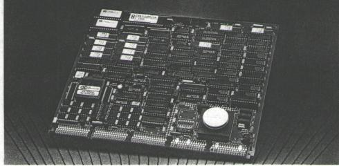
Shown above: CMD's CBI-1000/TM multi-function disk and tape VAXBI SCSI host adapter. Includes full support of multi-hosting across DEC buses as well as CMD software enhancement programs.
