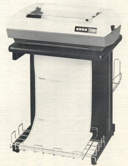
Quantex's 6010 dot-matrix impact printer operates at 150 cps with a 9 x 9 matrix and is microprocessor controlled.
