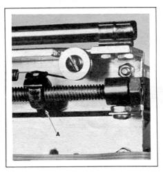
PHOTO 4: Close-up of the end of the drive screw, including the limit switch trip lever (A) and the drive nut connection arrangement. The reference pot is shown in the full reset position.
