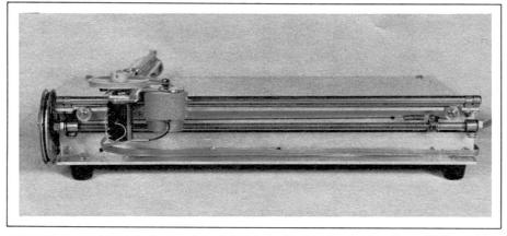
PHOTO 2: Front view of the pen carriage drive mechanism and pen servo motor, with the position reference pot in the reset position. Overall length is 13 inches.
