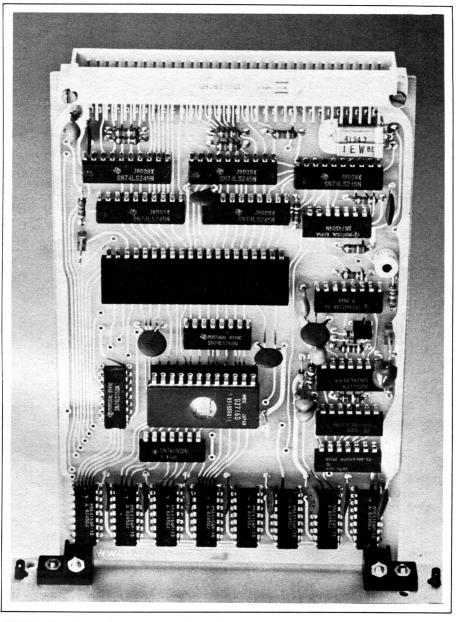
PHOTO 2: Since the size of system memory is largely determined by the processor, the author decided to integrate memory into the processor board. Doing so also eliminated the need for an extra Eurocard.
