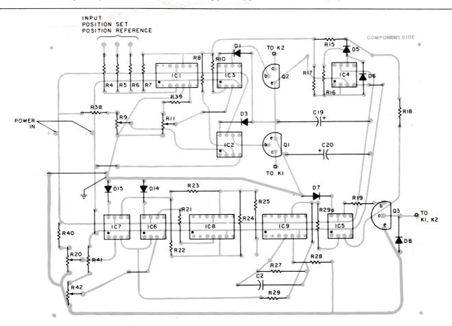
FIGURE 9: Stuffing guide for the servo circuit. Note that R42 is optional. See text.
