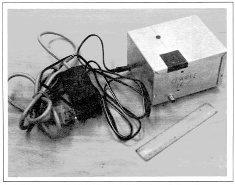
FIGURE 6: You can mount the RGB modulator in a mini-box and use a plug-in transformer to power it. The ruler is 6 inches long.
