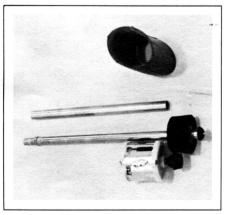
FIGURE 5: Partially assembled tool with the driven wheel on the shaft.
