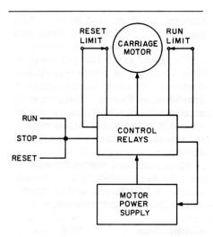
FIGURE 6: Block diagram of the direction-control circuit.
