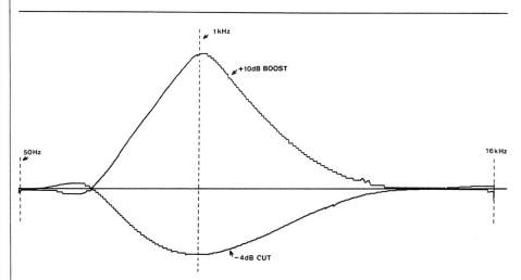
FIGURE 11: Complete system-frequency plot of a five-band equalizer set alternately for boost and cut. Shown at approximately one-balf scale.
