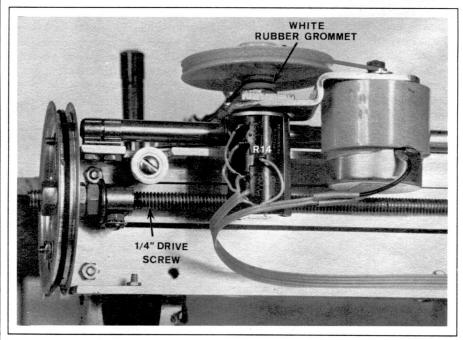
PHOTO 7: Low-angle front view of the pen motor/drive pulley and the dial string for the pen drive. Also shown is a soft, white grommet and a mounting clip for the pen carriage guide rod.
