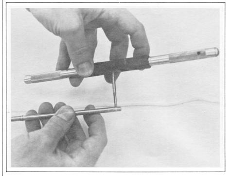
FIGURE 6: Run a #4-36 tap as far as it will go into the set screw hole.
