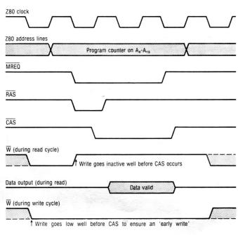
FIGURE 2: Timing for an op-code fetcb. The Z80 microprocessor bas a special register for use with dynamic RAMs, which provides a refresh address coinciding with a refresh control signal.
