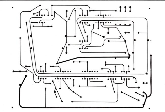
FIGURE 8: Circuit board pattern for the servo circuit. Enter Fast Reply #859 if you are interested in buying the board (estimated cost, \$9.50).
