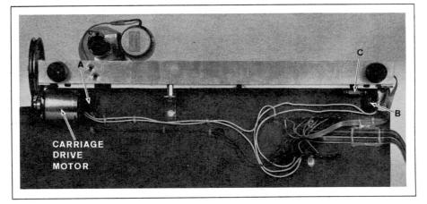
PHOTO 5: Bottom view of the pen carriage, drive motor, wiring and limit switches. A is the run limit, B is the reset limit, and C is the trip lever attached to a nut on the drive screw.
