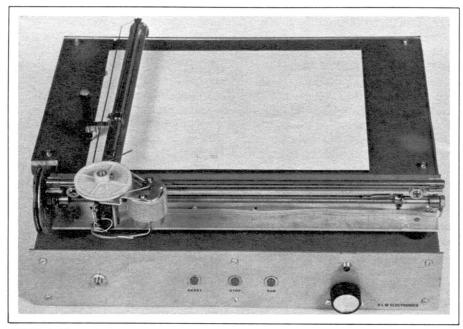
PHOTO 1: The author's chart recorder is built in two separate sections. The upper one bouses the mechanics and the lower one the electronics.
