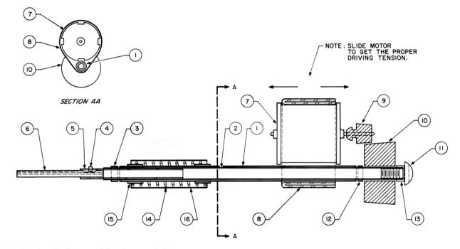
FIGURE 2: Schematic diagram of the wire-wrap tool.
