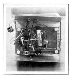
FIGURE 3: Wiring layout is not critical. The 'rat's nest'' technique used for the prototype proves this.
