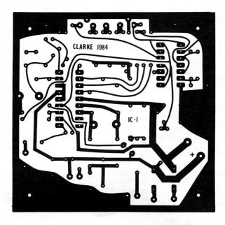
FIGURE 4: Board pattern for the RGB modulator circuit.
