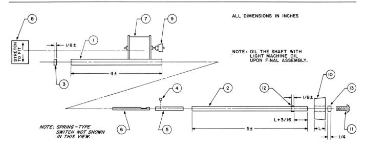
FIGURE 3: Exploded view of the tool's assembly.
