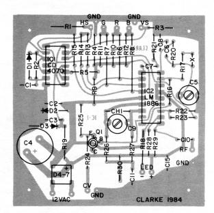
FIGURE 5: Stuffing guide for the modulator circuit.
