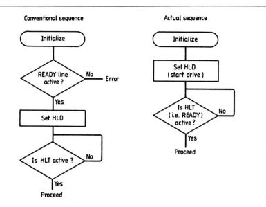
FIGURE 6: Floppy-disk controller read/write execution sequence.
