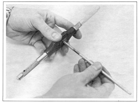
FIGURE 4: Run a #10-32 tap in the drive wheel end of the rotating shaft.
