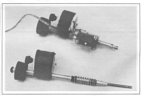
FIGURE 7: Although Mr. Neely used a spring switch (below), you might choose a micro switch (above).
