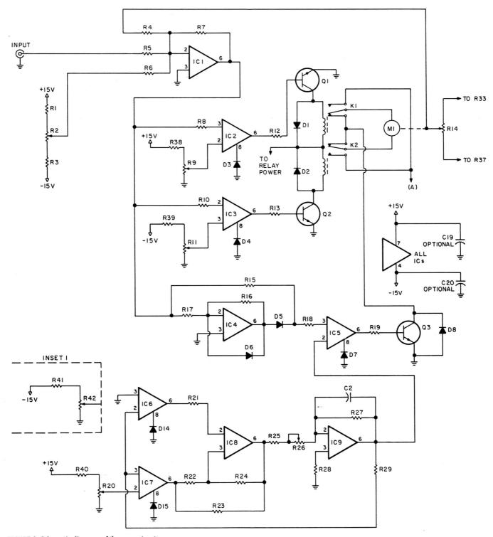
FIGURE 2: Schematic diagram of the servo circuit.
