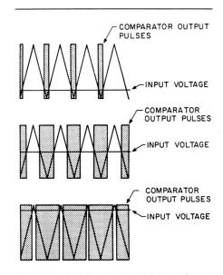
FIGURE 5: In pulse width modulation, the output pulse width is a function of the time between the crossings of the triangle and the modulating voltages.
