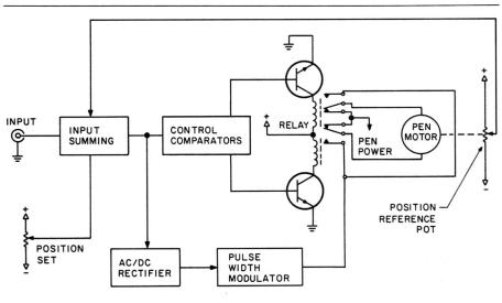
FIGURE 1: Block diagram of the servo circuit.
