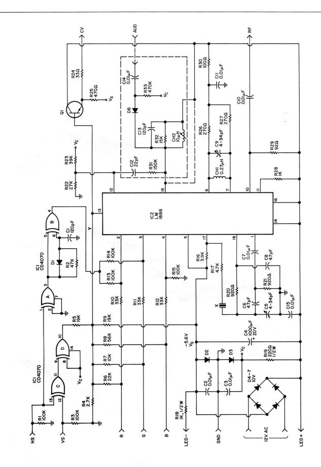
FIGURE 1: This circuit converts RGB output to a composite signal and provides an RF signal suitable for reception by a color TV.
