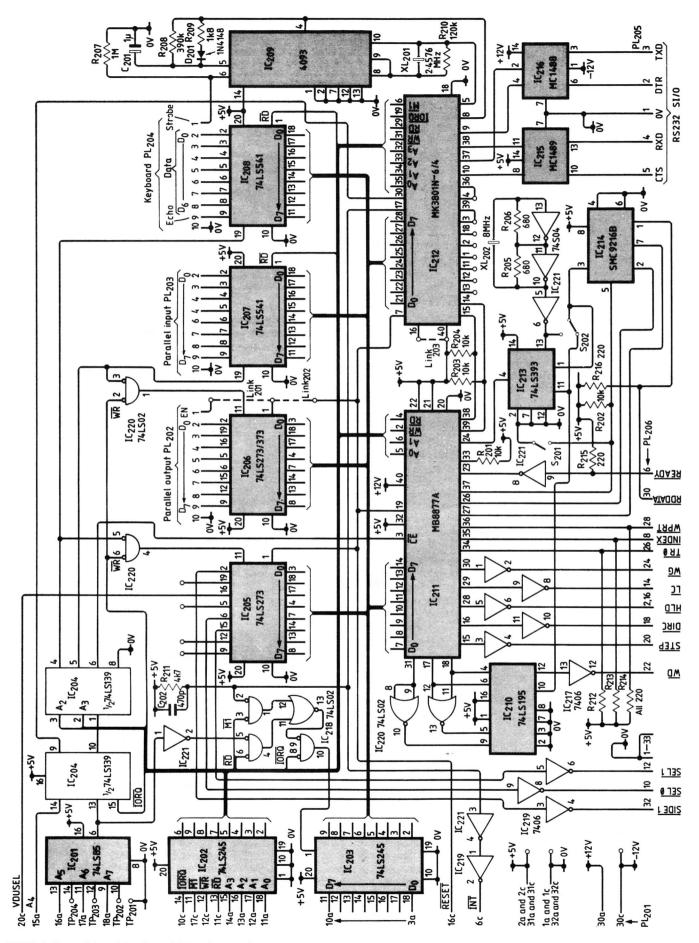
FIGURE 4: Floppy-disk, serial and parallel input/output (1/0) are provided on the 1/0 board. The beart of the circuit is the 3801, which contains a parallel port, a usart for serial communications, four counter/timers and an interrupt controller.
