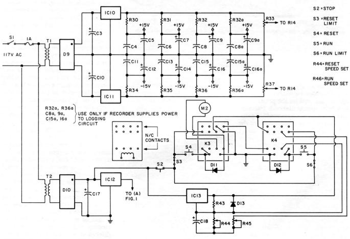
FIGURE 7: Schematic diagram of the direction-control circuit and power supply.
