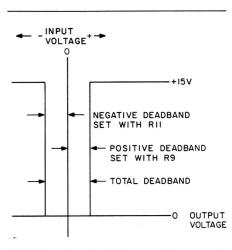
FIGURE 3: Operational diagram of the servo circuit's first stage.
