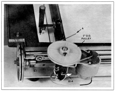
PHOTO 6: Top view of the pen bolder, pen lift wire (A) and slide construction. The diameter of the drive pulley is 2 inches, while the Plexiglas writing surface is ¼ inch thick. The pen is a fine-point marker that has been cut off.
