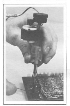
FIGURE 9: Wire-wrapping is a fast means of prototyping that allows you to make changes during the circuit assembly process.
