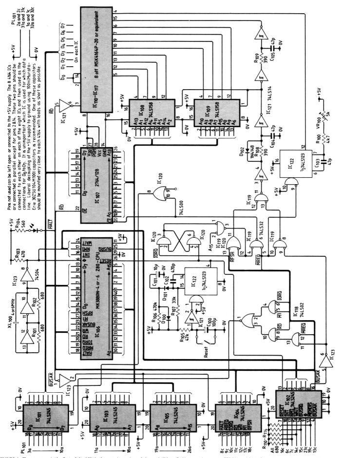
FIGURE 1: The processor is the first of the SC84's three main sections. It has a 64K-byte RAM, operating system EPROM and logic for a dynamic RAM, a hus driver and a reset control. On resetting, part of the ROM content is loaded into high RAM, and the ROM is then switched out, leaving up to 64K bytes for user programs.
