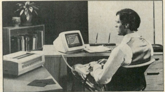
Digital Equipment Corp.'s Rainbow 100 personal computer. The LA50 dot matrix printer, shown at left, is one of three printer options.
