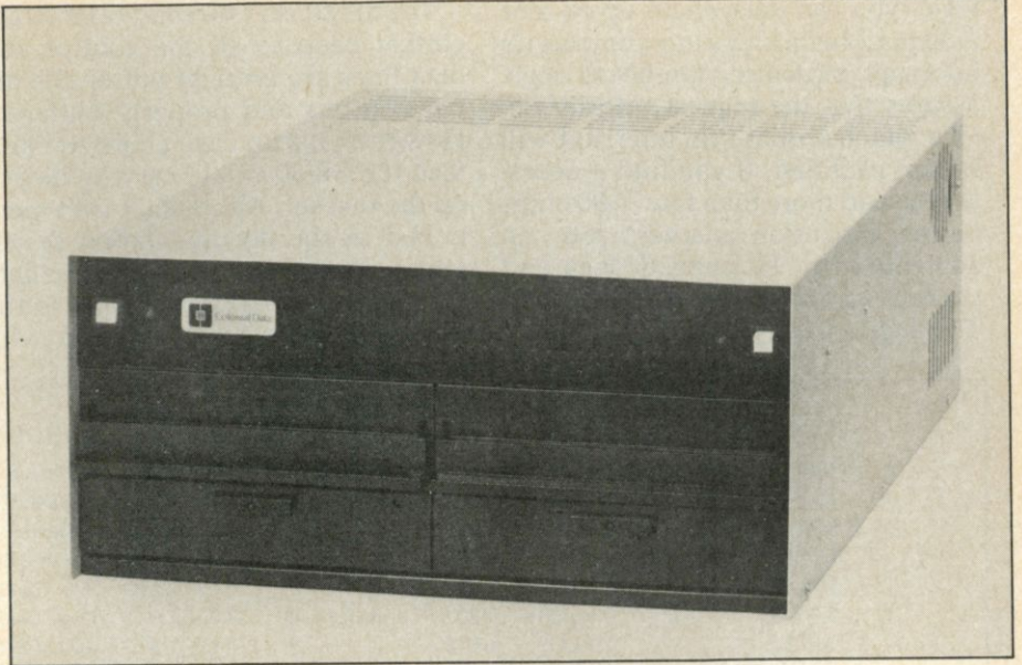
Colonial Data's single-board Z-80 computer, the SB-80.
