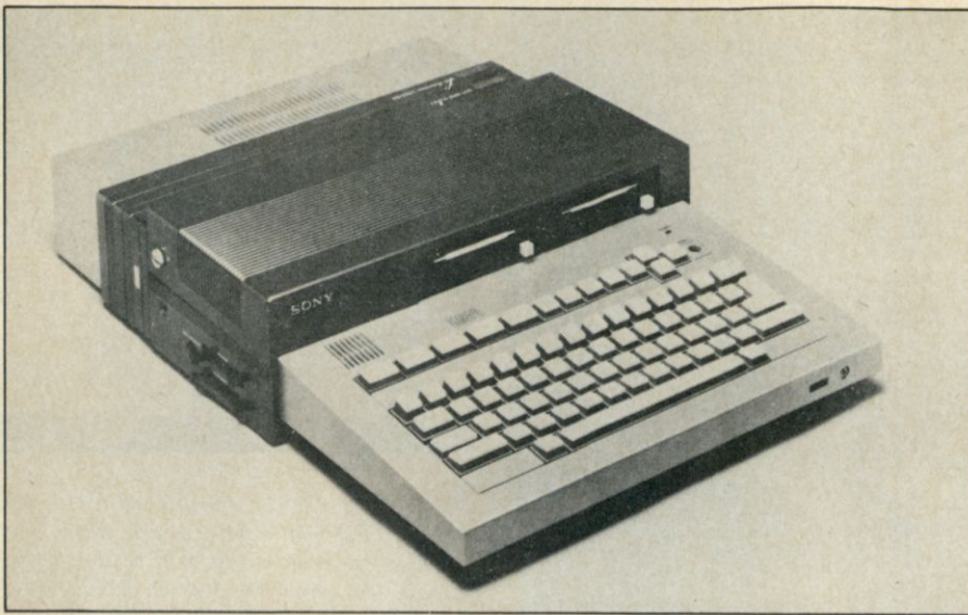
This is the new Sony SMC-70 microcomputer that was released at the National Computer Conference in Houston. In this photo, two 3 1/2-inch microfloppy disk drives and an expansion module have been mounted on the basic computer. The SMC-70 is a Z-80A microcomputer with 64K of RAM. Standard interfaces include a Centronics parallel printer port, an RS-232C serial port, RGB color and black and white composite video, light pen port, key pad interface and tape cassette I/O. In this configuration, with the disks, the unit would sell for about $2600.
