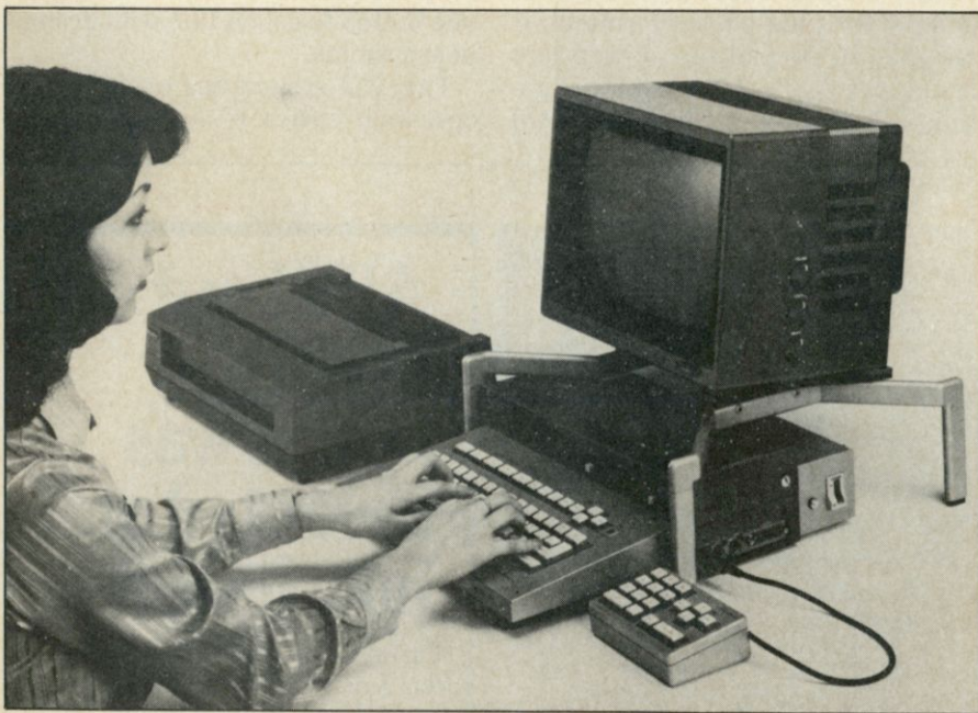
This is a typical business configuration of the SMC-70. A dot matrix printer, numeric keypad, monitor and 3 1/2-inch floppy disk drives have been added to the basic computer. The Sony green screen monitor sells for $375. A color monitor capable of accepting either RGB or composite video sells for $895. The monitor stand is another $60.
