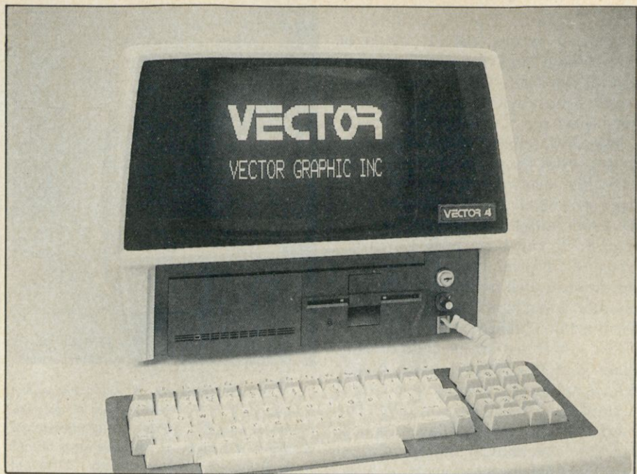
The Vector 8/16-bit microcomputer allows present and future software compatibility. The new Vector 4 offers a choice of several popular operating systems, and calls on 16-bit commands to significantly speed up selected eight-bit operations. Vector 4 is a product of Vector Graphic, Inc., Thousand Oaks, CA.
