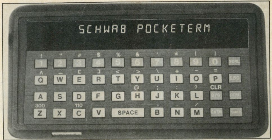
The Pocketerm is distributed by Charles Schwab & Co., best known as a firm of discount brokers. It is a portable terminal with a built-in modem. It provides either 110 or 300 baud communications service, and retails for about $400.
