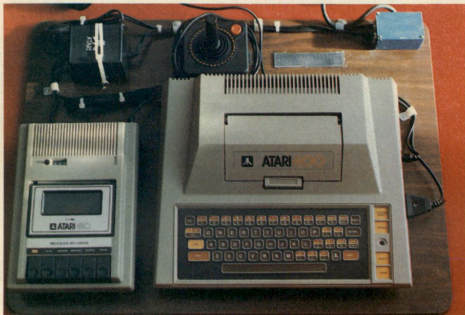
Photo 1. I've mounted computer, recorder, power supply and cables firmly to the board. The joysticks attach with Velcro.
