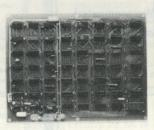
Non-destructive curser . Curser inputs: up, down, left, right, home, EOL, EOS • Scroll up, down • Requires +5 volts at 1.5 amps, and -12 volts at 30 mA • All 7400, TTL chips . Char. gen. 2513 . Upper case only . Board only \$39.00; with parts \$145.00
