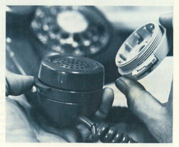
A hold button cuts noise on the line during data transfers. The unit in the photo is marketed under the name "Phone Censor" and is easy to install between the microphone and the handle.
