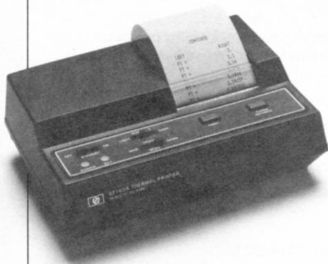
This HP-IL compatible printer/plotter automatically centers and justifies text to the left or right. It has numeric upper- and lowercase alpha, double-wide characters, and intensity control for optimum contrast and readability. Additionally, it supports STANDBY mode that lets any HP-IL controller on the loop manage its power consumption.
