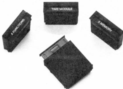
\*No more than one HP 82180A Extended Functions/Memory Module or two HP 82181A Extended Memory Modules should be plugged into an HP-41CV. The HP 82180A is required when using the HP 82181A.
