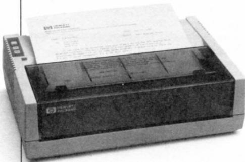
The 11 x 12 dot-matrix format text mode has a logic-seeking feature to find the fastest print route. Add a bold mode that won't slow printing speed to handle most of your letter-quality needs. A ROMAN8 character set provides 216 USASCII printable characters for use in many languages. Print on single sheets or fanfold paper.
