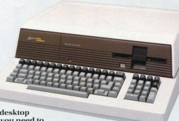
Built-in 5.25" floppy disk drive stores up to 320K bytes of data on a single disk; optional, external 8" disk drives can be added.
