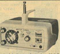
Designed for servicing the entire signal circuit system of any color or black & white television receiver by signal substitution. Substitutes these signal stages: VHF tuner, each video IF stage, video detector, video amplifier, 4.5 MHz sound IF amplifier, sound limiter, sound detector and audio amplifier. Also tests UHF tuner, antenna system and AGC system.
