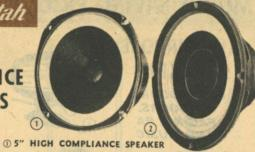
Outstanding base response in a small sealed enclosure makes this the perfect woofer for tiny bookshelf systems or other special speaker systems. Has enormous power handling capacity of 18 watts with its extra-heavy 10 oz. Ceramic magnet. Frequency response 65-17,000 Hz. Complete with design specifications for enclosure. 51/8" Dia. x 21/8" D. Shpg. wt. 2 lbs. \$11.95 34A493-7. Each .
