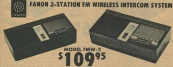
Ultra-quiet 2 channel, 2 station FM wireless intercom system for home, office and factory. Advanced phase-locked loop FM circuitry, blanks out hum, static and
