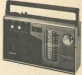
Features an FET RF amplifier. Built-in AFC for FM and squelch control for noise free PSB band. 3-5/8" speaker. Telescoping antenna for FM/PSB and ferrite bar AM antenna assure sensitivity on all bands. Has separate power, volume and tone controls and large, easy-to-tune vertical dial. Has earphone jack. Striking black and brushed metal case is 7-7/8 H. x 10 ½ W. x 3-3/8" D. Operates on 4 "C" cell batteries listed below or 120 V 60 Hz AC. Shpg. wt. 4 lbs.
