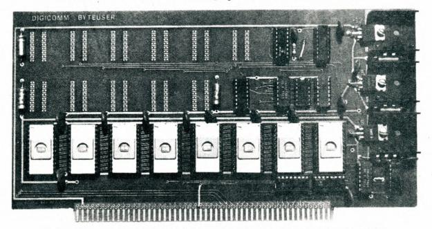
WORKSPACE ON BOARD FOR ELEVEN WIRE WRAP SOCKETS WHICH COULD BE USED FOR 1K RAM. VECTOR INTERRUPT KEYBOARD. INPUT/OUTPUT PORT, SIMPLE CASSETTE INTERFACE OR PROM PROGRAMMER.
