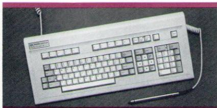
**KB 5152B** Add bar code with a plug-compatible keyboard for the IBM® PC, XT or AT. Installs fast and easy by plugging it in. Includes Key Tronic's professional series keyboard, engineered to increase operator productivity. Auto-discriminates and reads most popular bar codes. Scans forward or reverse for efficient operation.
