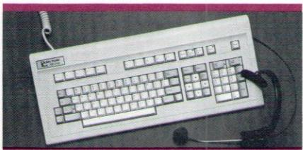
**KB 5152V** Use speech recognition to increase the efficiency of computer input by complementing your keyboard with the ability to respond to a human voice. No software modifications are needed because commands are presented to the computer like keyed input.
