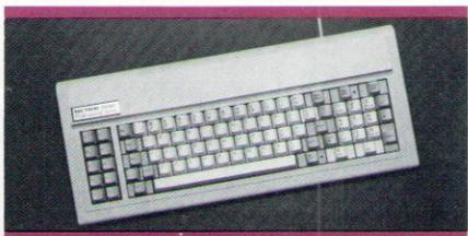
**KB 5150** Designed to make word processing faster and more convenient with your PC, XT or PCjr. Easy to use because SHIFT and RETURN keys are located in the same place as Selectric® keyboards and the ENTER key is separate to speed up data entry.
