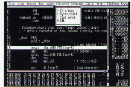
With Microsoft Macro Assembler version 5.1, you can now debug assembly-language programs written for the 80386, disassemble 80386 instructions, and display the extended 80386 register set.
