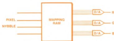
In nybble mapped operations each 4-bit nybble can select one of 4096 colors as determined by a mapping RAM. The contents of the mapping RAM can be changed dynamically, under software control, by issuing OUTPUT instructions to the SDI.
